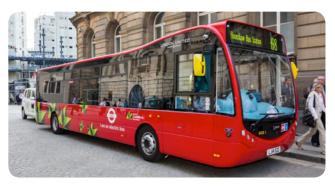
In York six Versa electric buses powered by Magtec drive train systems rolled into operation as York City Council officially opened its new Askham Bar and Poppleton Bar Park and Ride schemes.
